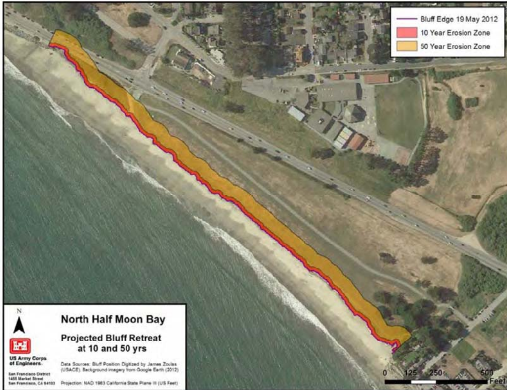
Figure 4. Extent of Projected Bluff Retreat at 10 and 50 Years (based on the estimated retreat rate of 1.64 ft/yr) Source: Lin et al. (2015).
